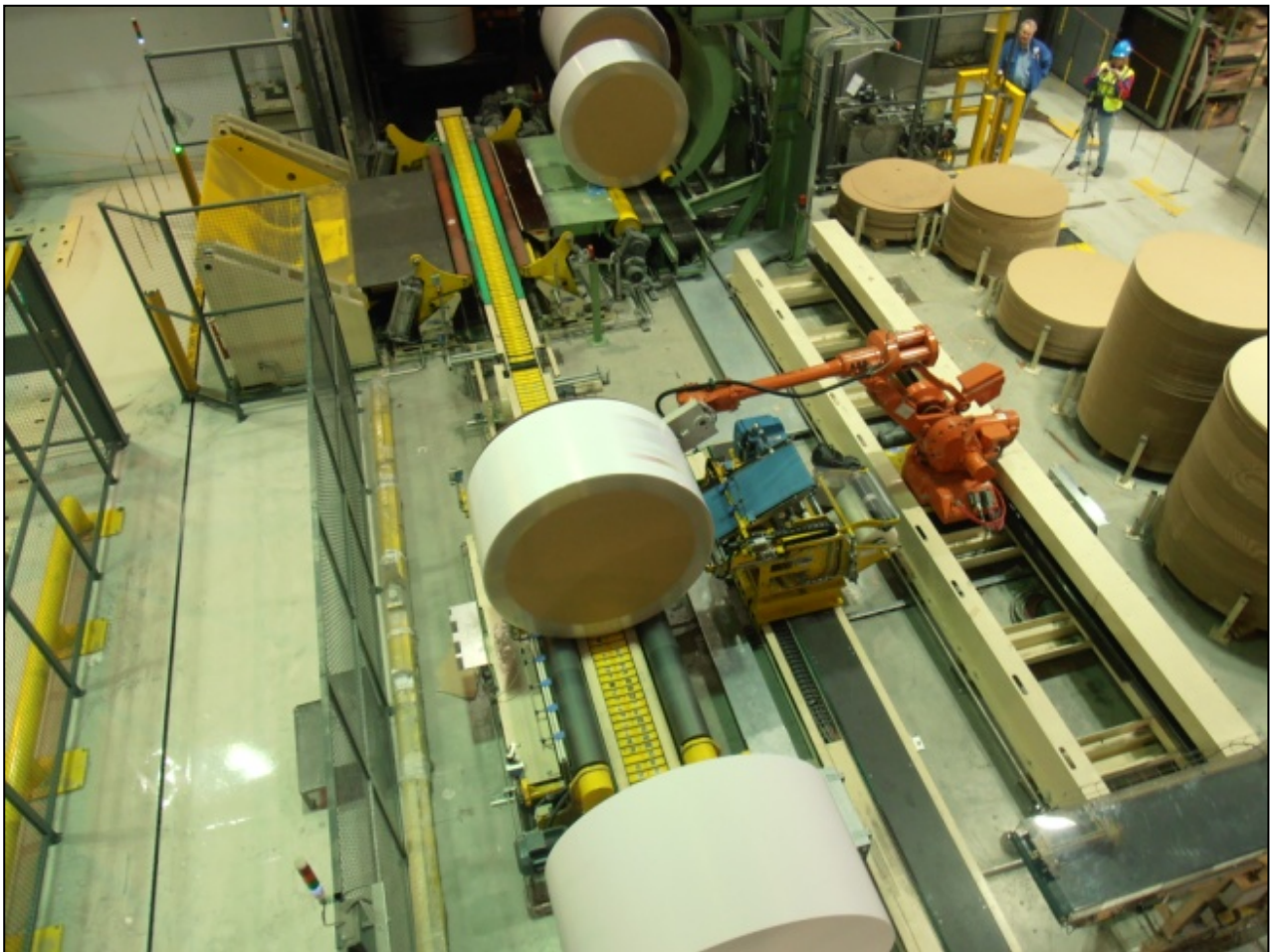
Figure 6 Fully automated stretch film packing in Metsä Board Äänekoski. Corrugated heads to protect the roll ends with radial stretch wrapping for the body and corners, and plain paper labels without glue slipped under the film layer.
