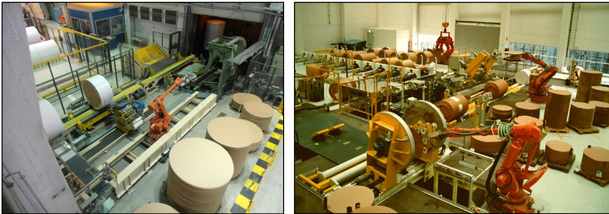
Figure 1 Paper roll packing methods can be divided to two main categories - stretch (on the left) and kraft wrapping (on the right). 图 1: 纸卷包装方式主要有两种—缠绕包装（左图）和牛皮纸包装（右图）
